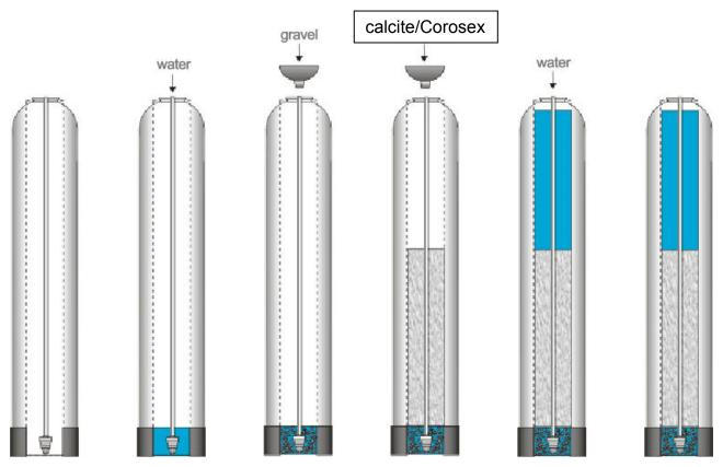
Once you have finished adding the media to the tank, remove the tape from the distributor tube. Be careful not to pull upwards on the riser tube while doing this as it is important that the distributor remain in its recess at the bottom of the tank.
